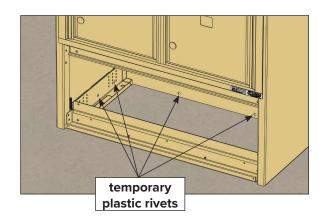
Remove the two mounting brackets and two skirt plates from the cabinet, and set them aside for later installation.
