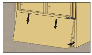
Remove and discard the plastic push-in rivets which hold the two mounting brackets and two skirt plates in place inside the lower compartment of the 4C Depot cabinet.
