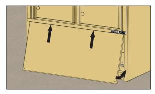
2 • Secure the lower-front panel to the cabinet using a #2 square-tip 1/4" hex-shank insert driver bit and the two (2) screws removed at the start of the installation.
